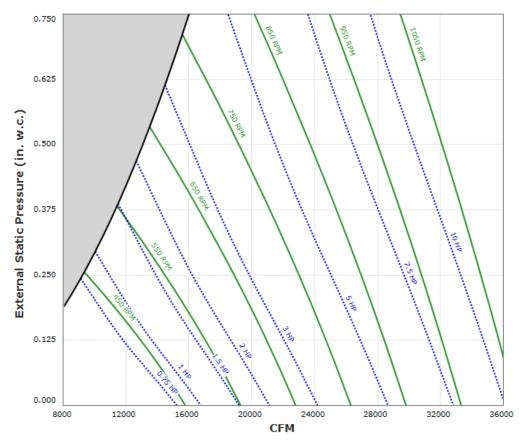
Max Sizeable RPM = 1050 RPM. Curve shown extended beyond this point for reference only.
